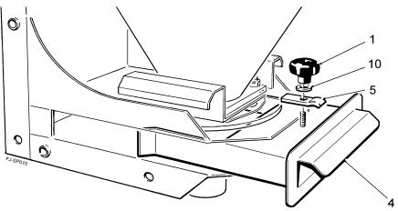
1. Place the chute (item 4) between the top and bottom plates of the Fan Jet chassis, with the threaded stud for the clamp positioned centrally in the recess, against the outer edge of the top plate. Then fit the flat washer (item 10) Ensure it is positioned square to the chassis and tighten the retaining plate clamp (5) using the threaded knob (1) to hold the chute firmly onto the machine.
