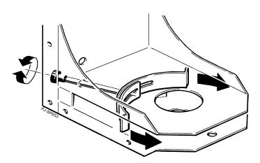
The machine has two adjustable sliding deflectors that fit around the disc and are used to physically limit the throw of material off the disc in order to adjust spread width and pattern, either equally to both sides or as a border control to one side only.
