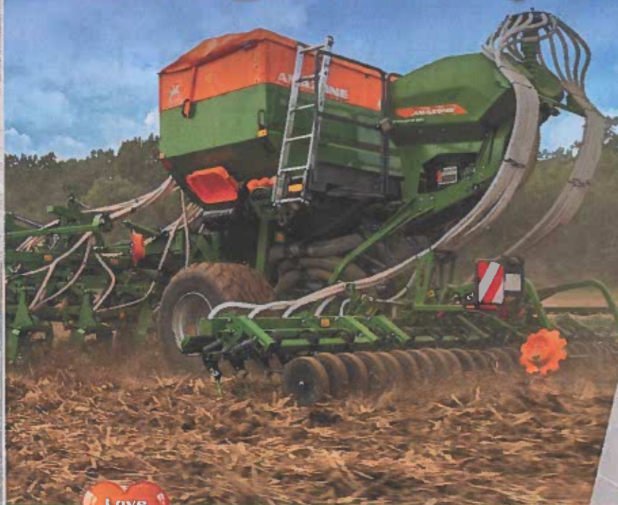
Each individual hard-faced chisel opener is guided at the perfect planting depth by the following Reflex rollers.
