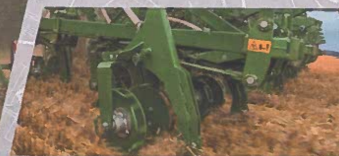
Each individual hard-faced chisel opener is guided at the perfect planting depth by the following Reflex rollers.
