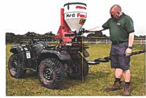
Ensure the pelleter is at the correct height and tilted at the right angle so that it reaches the desired spread width.
